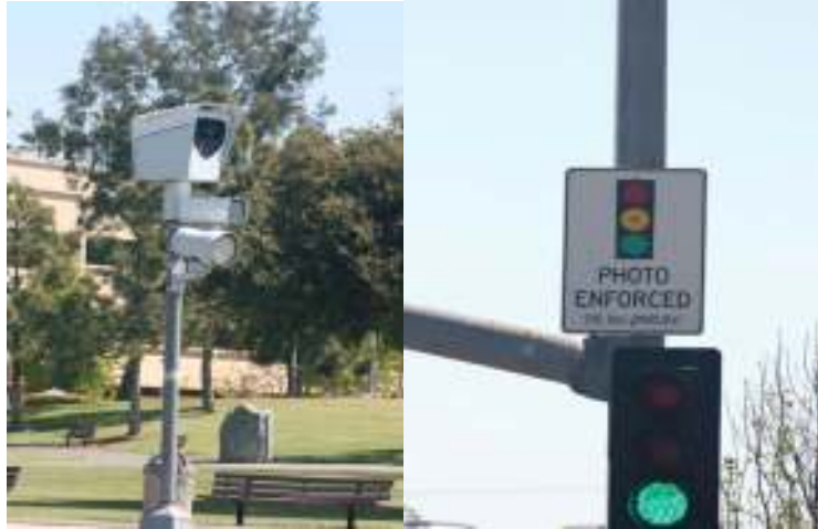
Typical Red Light Camera installed in Ventura
