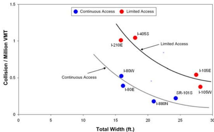
Figure 6 Relationship between total width and collision rate.
