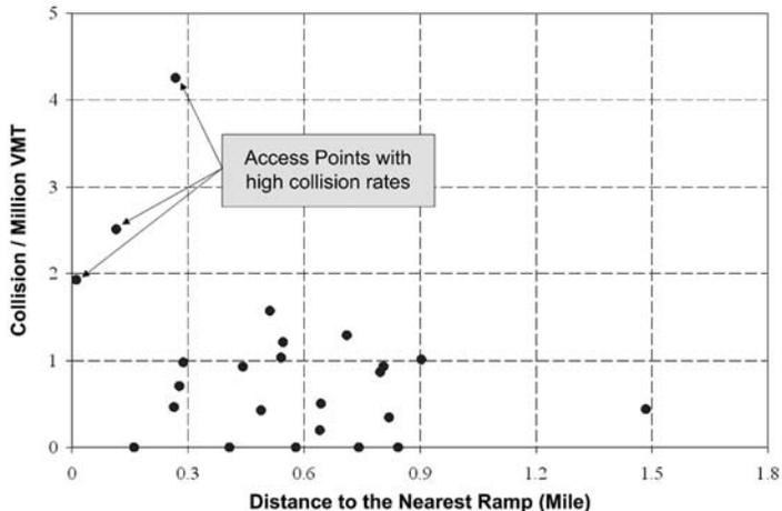
Figure 7 Relationship between collisions per mile per hour and distance to nearest entrance/exit ramp in limited access HOV facilities.
