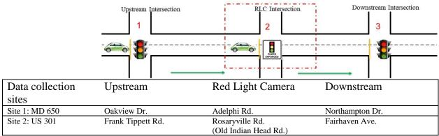
Figure 6: Graphical Illustration of Field Data Collected in Stage-I
