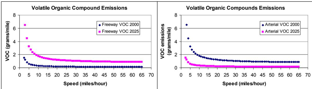
In addition to these “steady speed” emission rate values, emissions tend to be highest during acceleration. Engine operation is less efficient during these times and more unburned fuel is sent through the exhaust system.
