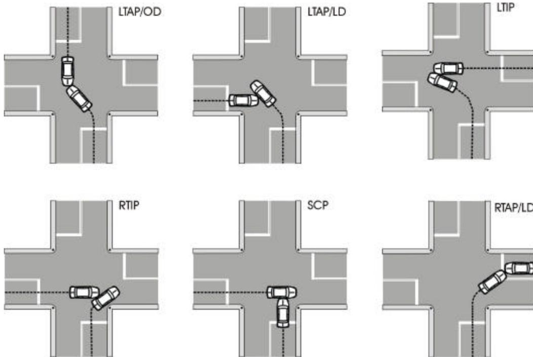
**Figure 28: Schematics of Common Crossing Path Crash Scenarios (7).**
